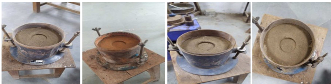
Figure 5. Soaked and Un-soaked CBR samples.
