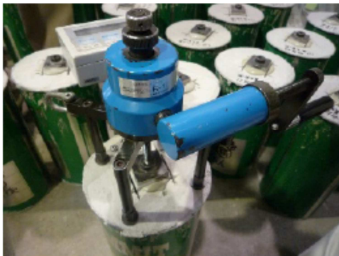
Figure 3. View of surface tensile test.
