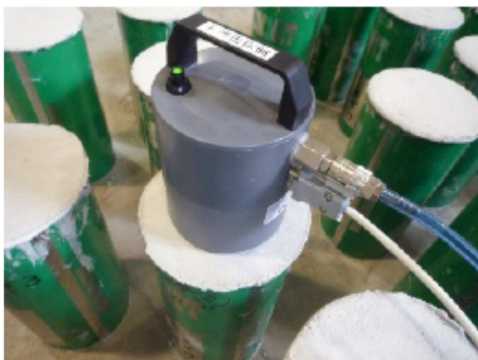
Figure 4. View of air permeability test.
