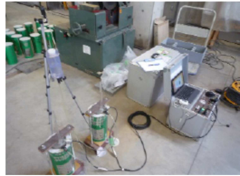
Figure 5. View of water absorption test.
