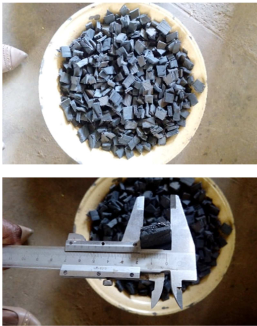
Figure 1. Coarse rubber aggregates obtained from used tyres.
