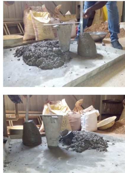
Figure 2. Slump of normal and Rubberized Concrete.
