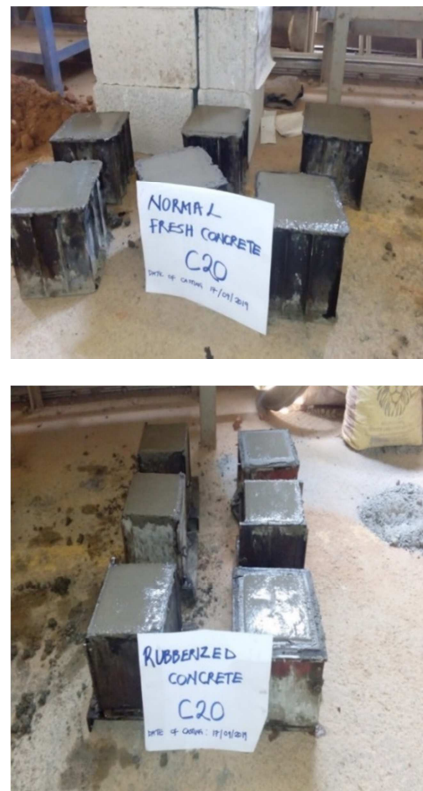
Figure 3. Casting of control and rubberized concrete specimens.
