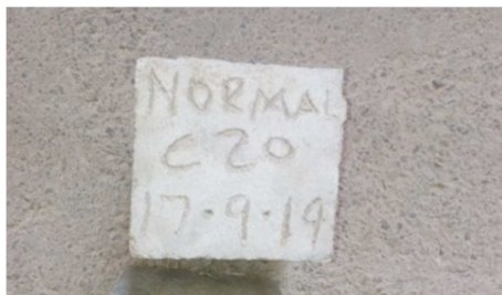
Figure 8. Rubber reinforced concrete and normal concrete exhibiting some cracks after being subjected to heat at 100°C for 48 hours.
