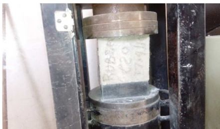
Figure 8. Rubber reinforced concrete and normal concrete exhibiting some cracks after being subjected to heat at 100°C for 48 hours.
