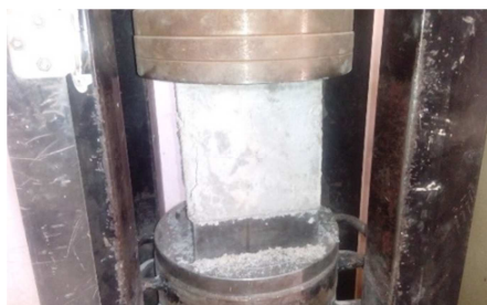
Figure 9. Compression test of heated rubber reinforced concrete.
