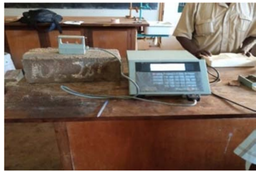
Figure 2. Determination of thermal conductivity of the blocks.
