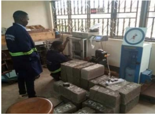
Figure 1. Determination of compressive strength of the blocks.
