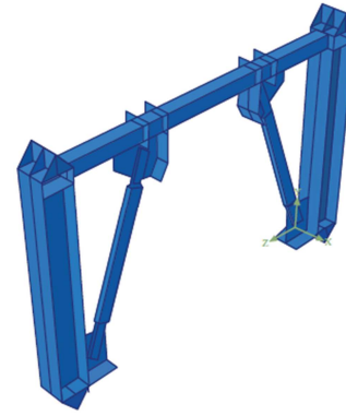
Figure 6. BRBF with moment link [25].
