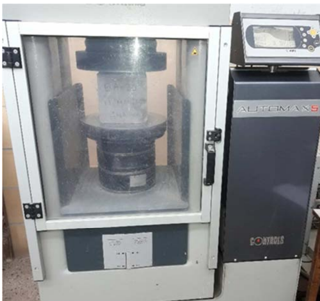
Figure 5. Compressive strength test.
